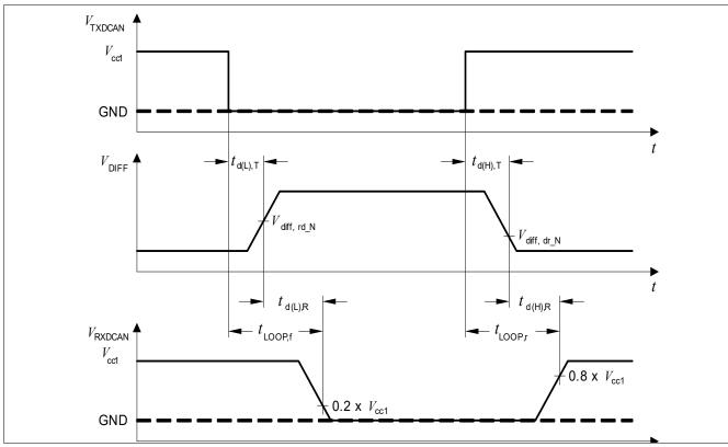
Figure 28 Timing Diagrams for Dynamic Characteristics
