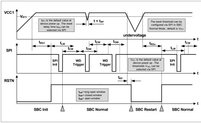
Figure 37 Reset Timing Diagram
