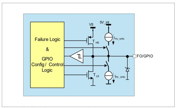
Figure 35 Simplified Fail Output and GPIO Block Diagram
