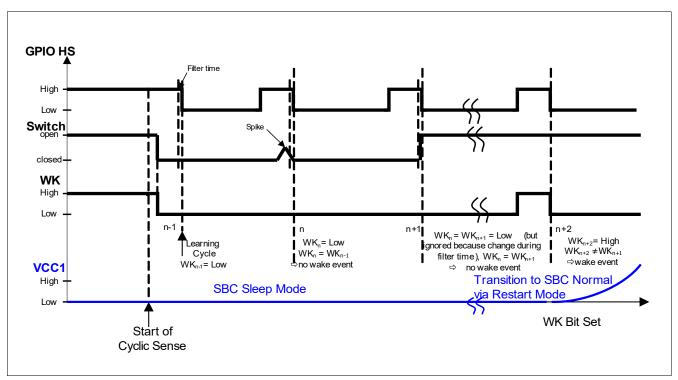
Cyclic Sense Example Timing for SBC Sleep Mode, HS starts with On, Figure 10 **GND based WK/VSENSE input**
