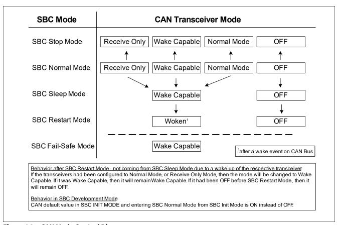
Figure 24 CAN Mode Control Diagram
