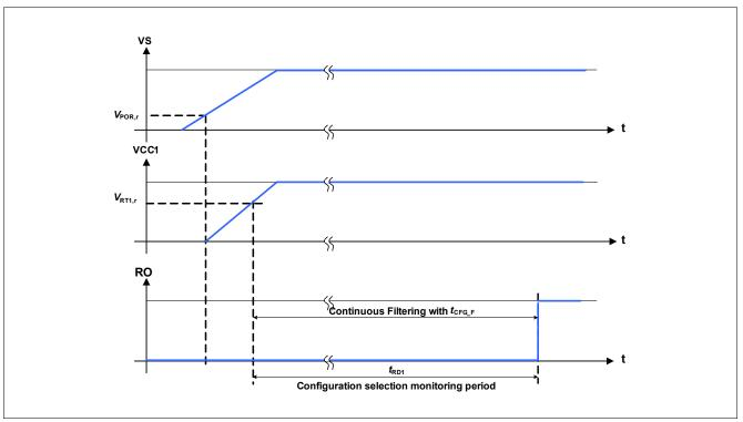
Figure 4 Hardware Configuration Selection Timing Diagram
