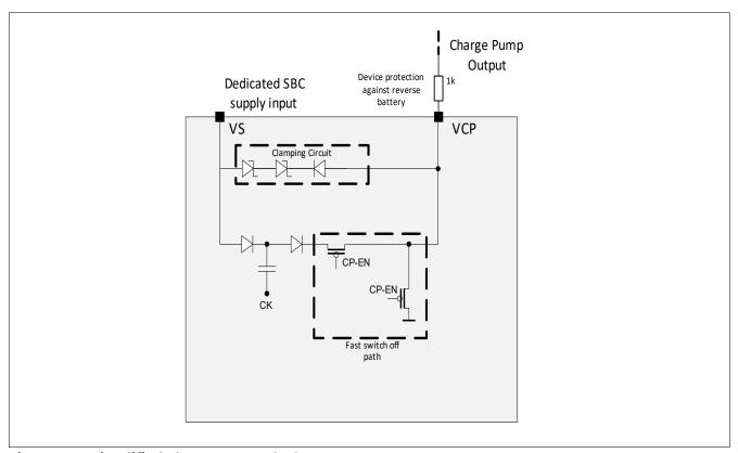
Figure 12 Simplified Charge Pump Block
