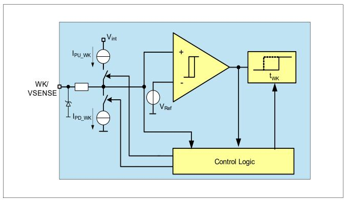
Figure 30 Wake Input Block Diagram
