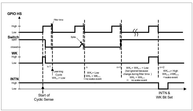
Cyclic Sense Example Timing for SBC Stop Mode, HS starts Low, GND based WK/VSENSE Figure 9 input
