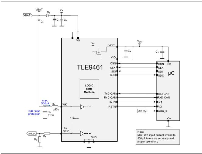
Figure 52 Simplified Application Diagram showing the Alternative High-Voltage Measurement Function via WK/SENSE and FO/GPIO
