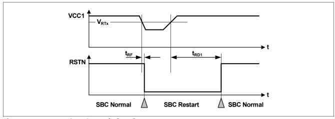
Figure 42 VCC1 Undervoltage Timing Diagram
