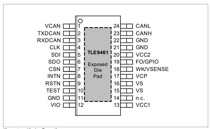
Figure 2 Pin Configuration
