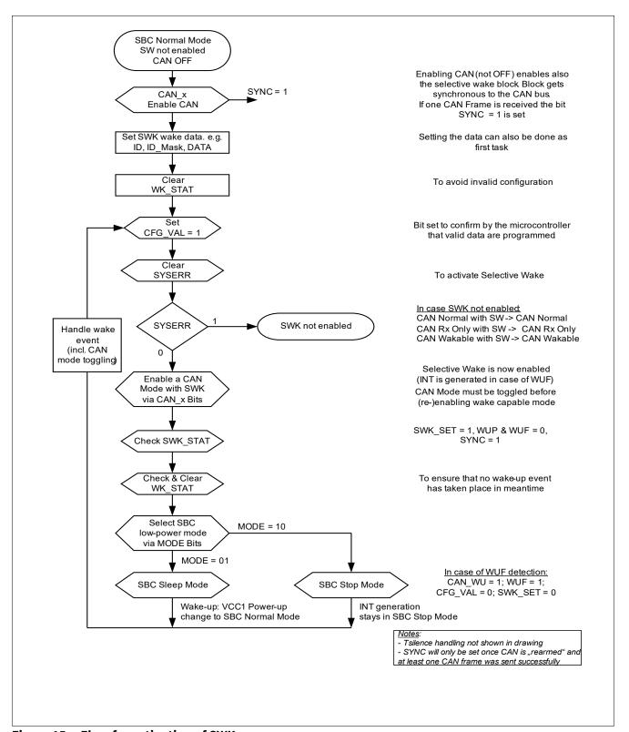
Figure 15 Flow for activation of SWK
