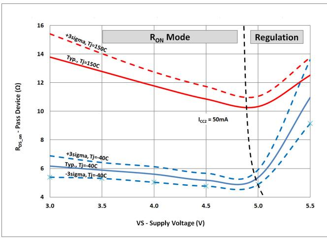
Figure 22 On-resistance range of VCC2 pass device during linear ( $R_{ON}$ ) mode for  $I_{CC2}$  = 50mA
