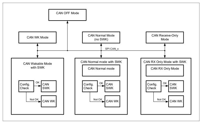
Figure 17 CAN SWK State Diagram
