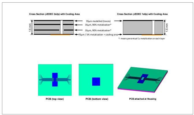
Figure 55 Board Setup
