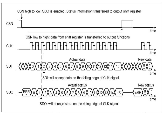
Figure 44 SPI Data Transfer Timing (note the reversed order of LSB and MSB shown in this figure compared to the register description)
