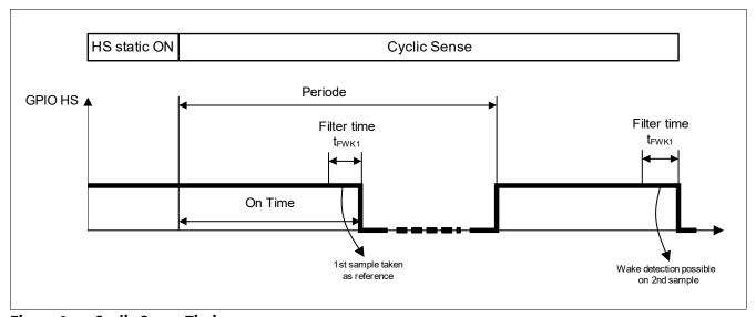
Figure 8 Cyclic Sense Timing
