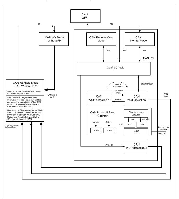
Figure 14 CAN Selective Wake State Diagram
