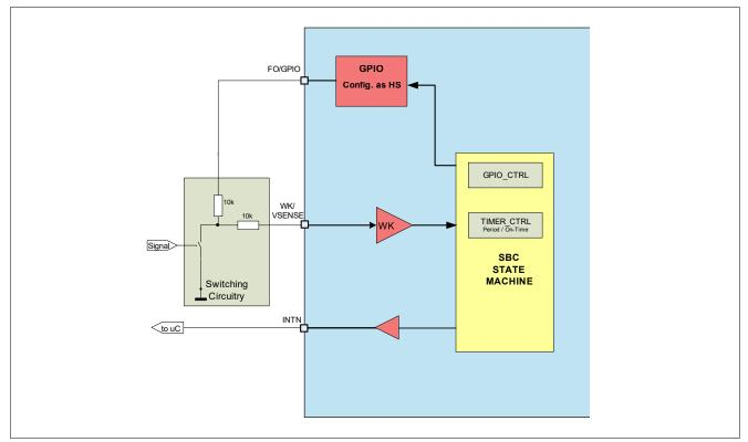
Figure 6 Cyclic Sense Working Principle
