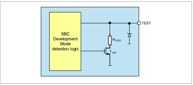
Figure 5 Block Diagram of Pin TEST for SBC Development Mode Detection
