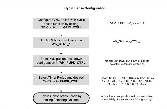
Figure 7 **Cyclic Sense: Configuration and Sequence**
