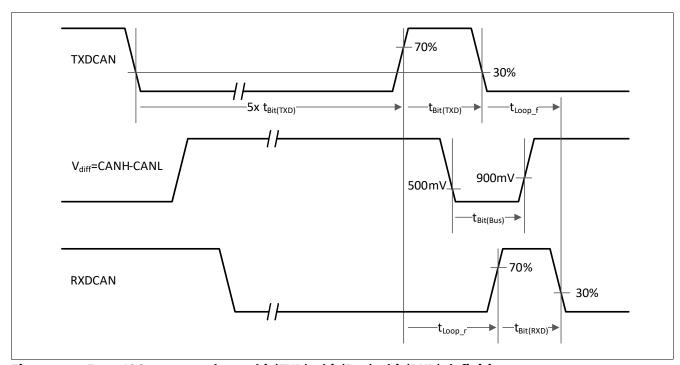
Figure 29 From ISO 11898-2: tloop, tbit(TXD), tbit(Bus), tbit(RXD) definitions
