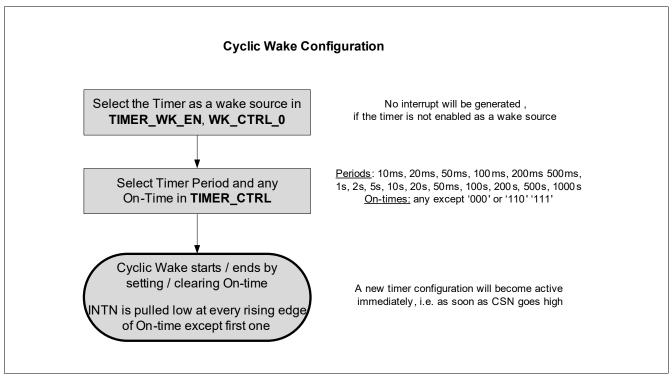
Figure 11 Cyclic Wake: Configuration and Sequence
