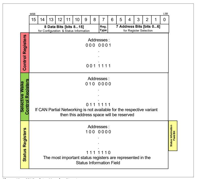
**SPI Register Mapping Structure** Figure 47
