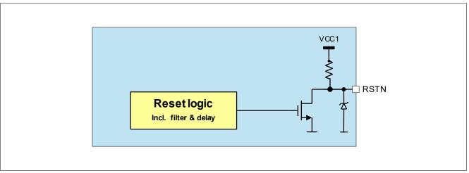
Figure 36 Reset Block Diagram
