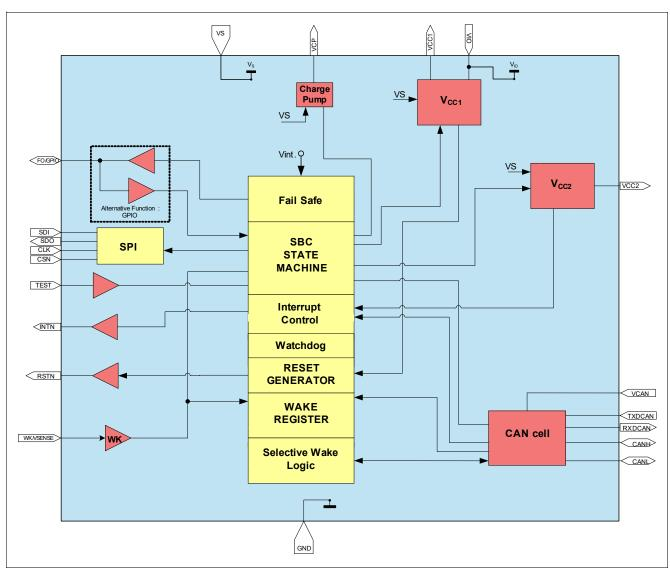
Figure 1 TLE9461-3ES V33 Block Diagram
