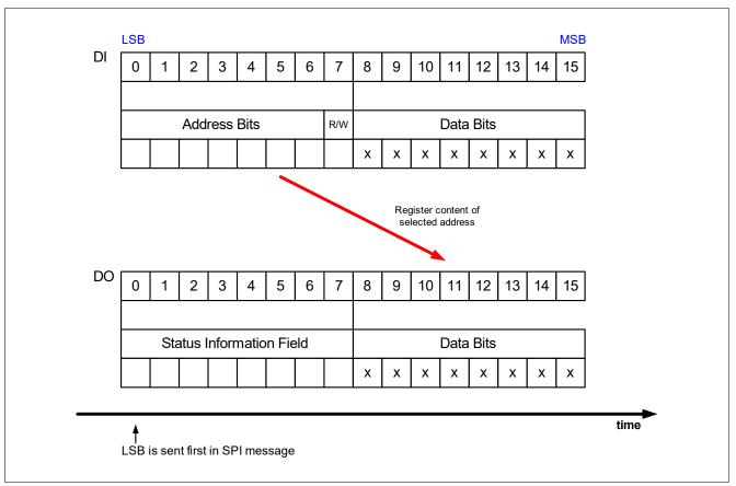
Figure 45 SPI Operation Mode
