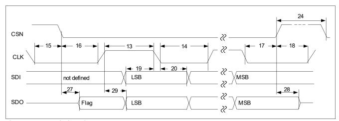
Figure 49 SPI Timing Diagram
