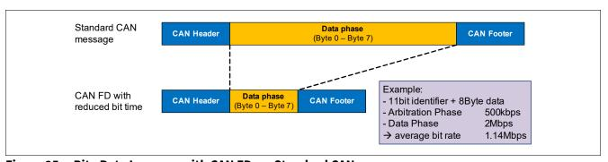
Figure 25 Bite Rate Increase with CAN FD vs. Standard CAN
