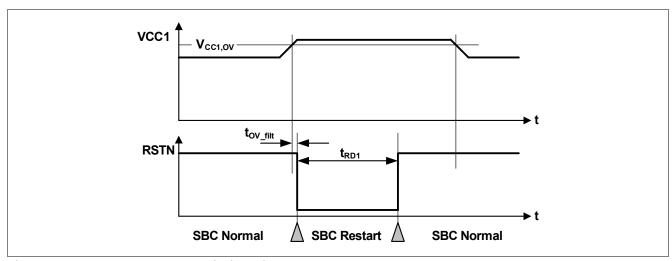
Figure 43 VCC1 Over Voltage Timing Diagram
