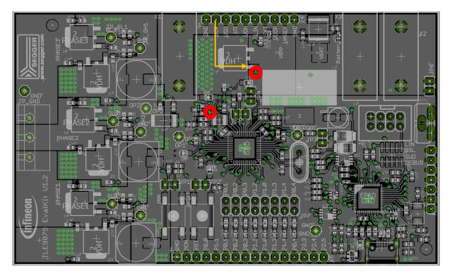
Note: The disconnected Transistor T1 can cause a voltage drop from VBAT connection to VDH voltage level. This voltage drop can be avoided by manually connecting the Gate Pin of T1 to the VCP voltage Pin (orange arrow).
