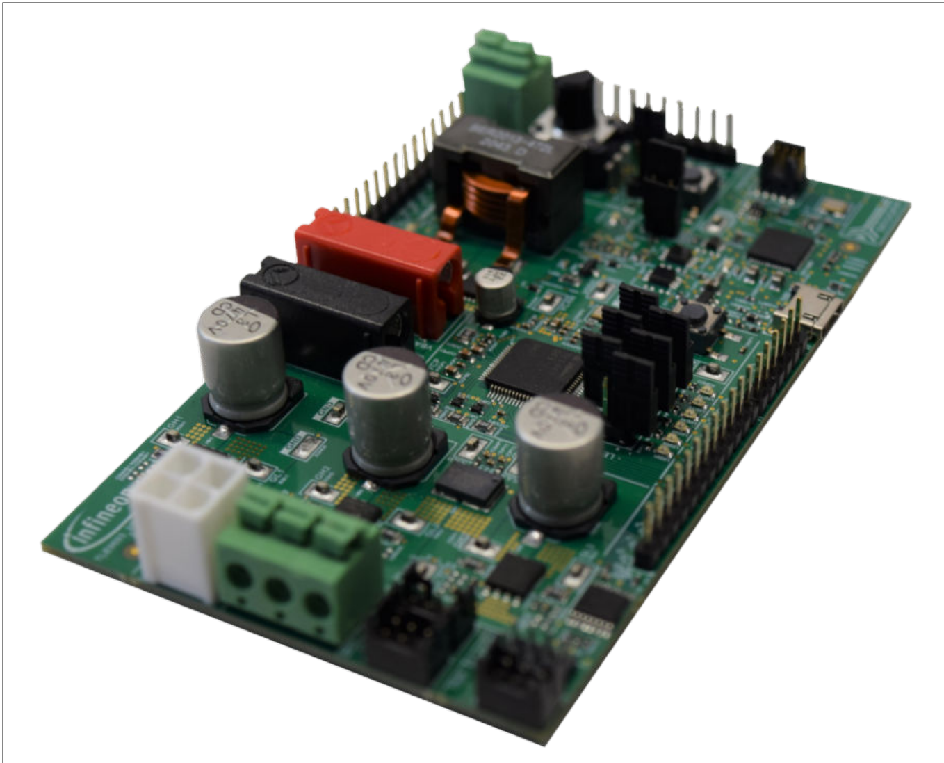
Figure 1 MOTIX™ MCU TLE9893-2QK evaluation kit
