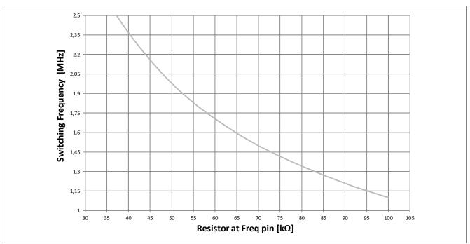
Figure 7 Switching frequency  $f_{OSC}$  versus frequency setting resistor  $R_{FREO}$ .
