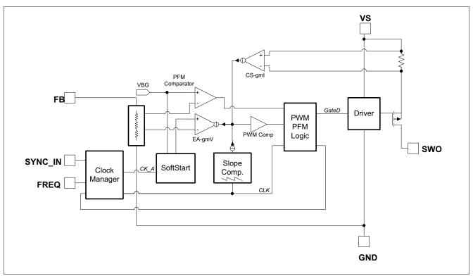
Figure 3 Block diagram buck regulator
