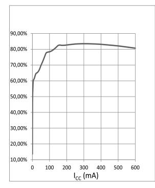
Efficiency for  $V_{\rm S}$  = 13 V,  $f_{\rm OSC}$  = 2.2 MHz,  $L_{\rm OUT}$  = 4.7 µH
