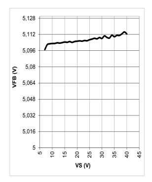
Line regulation PFM mode  $I_{cc} = 100 \ \mu\text{A}; T_J = +25^{\circ}\text{C}$
