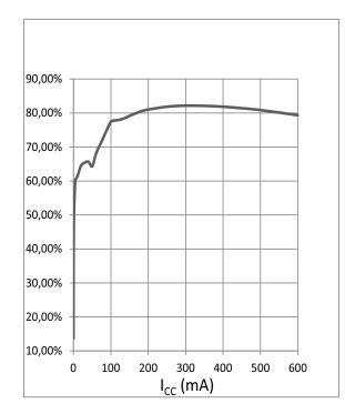
Efficiency for  $V_{\rm S}$  = 13 V,  $f_{\rm OSC}$  = 1.65 MHz,  $L_{\rm OUT}$  = 10  $\mu$ H
