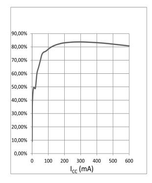
Efficiency for  $V_{\rm S}$  = 13 V,  $f_{\rm OSC}$  = 2.2 MHz,  $L_{\rm OUT}$  = 10  $\mu$ H
