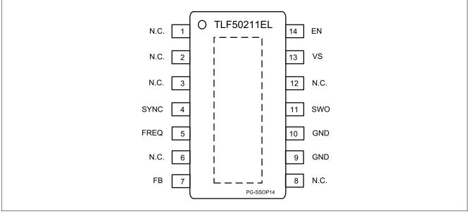
Figure 2 Pin configuration
