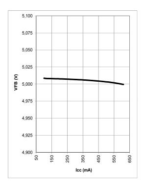
Line regulation PWM mode  $V_{\rm S} = 12 \text{ V}; T_{\rm J} = +25^{\circ}\text{C}$
