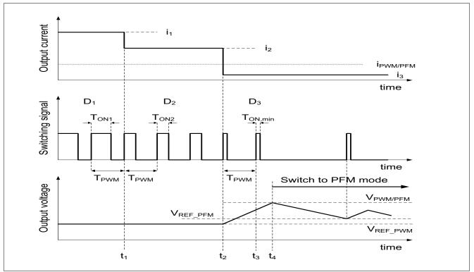
Figure 4 PWM to PFM transition (timing diagram)
