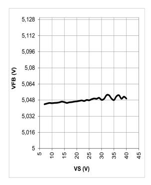
Line regulation PFM mode  $I_{cc} = 100 \mu A; T_{J} = +150^{\circ}C$
