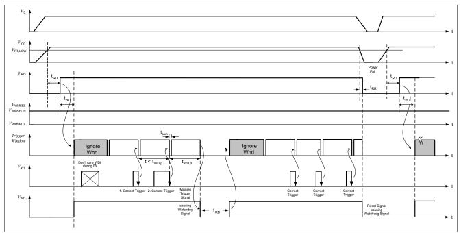
Figure 9 Watchdog timing diagram, slow watchdog timing
