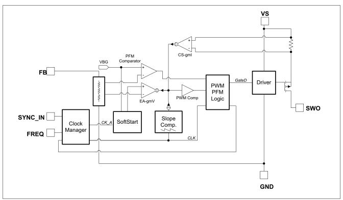
Figure 3 Block diagram buck regulator
