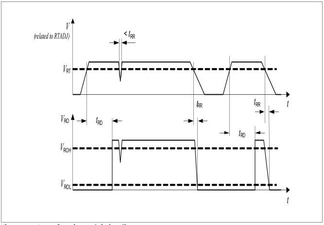
Figure 7 Reset function and timing diagram
