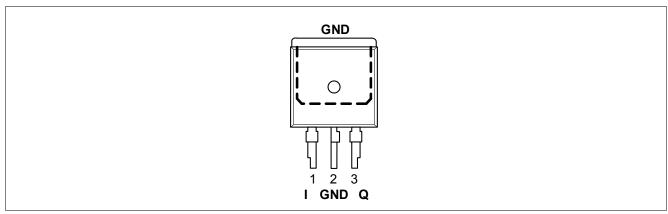
Figure 2 Pin Configuration
