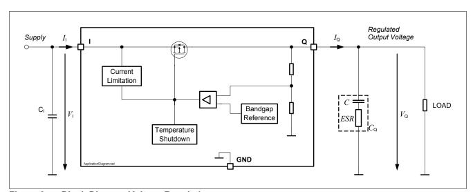
Figure 3 Block Diagram Voltage Regulation
