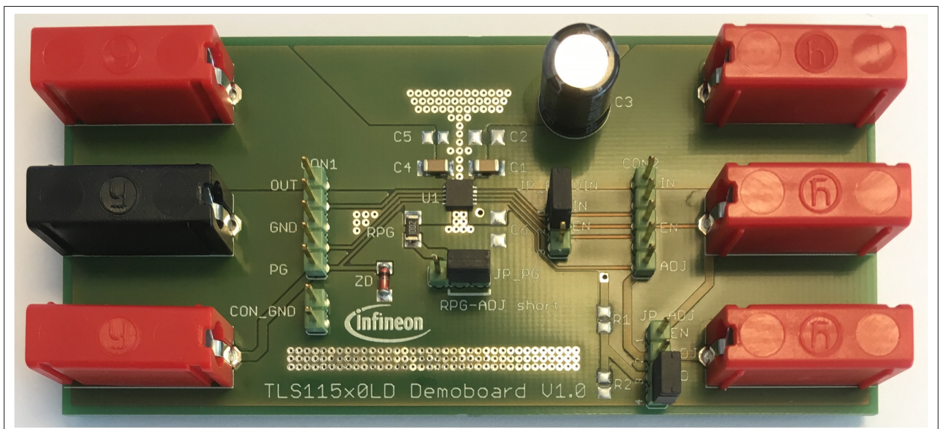
Figure 3 OPTIREG™ linear voltage regulator TLS115x0LD demoboard
