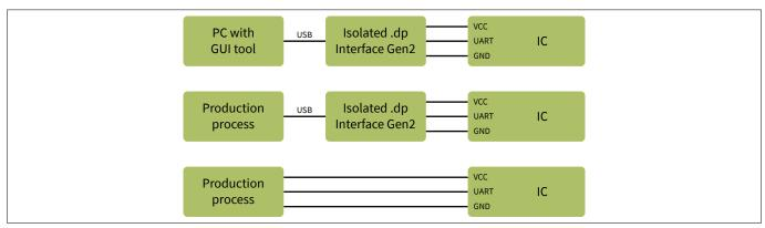
Figure 28 Setup for Parametrization using .dp Interface Gen2 for Interactive Development (top) and Production (middle and bottom)
