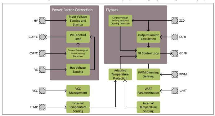
Figure 2 XDPL8220 Simplified Functional Block Diagram
