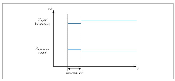
Figure 12 V<sub>in</sub> protections
