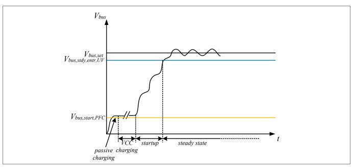
Figure 9 V<sub>bus</sub> Soft Start and Regulation
