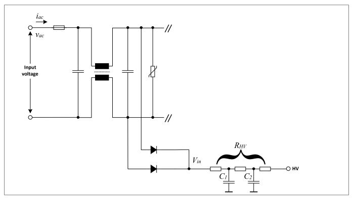
Figure 8 **Input Voltage Sensing Schematic**
