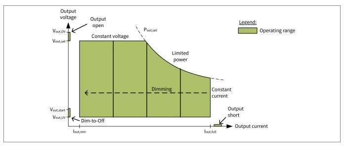
Figure 18 Control Scheme for CC/CV/LP Modes (including Dimming)
