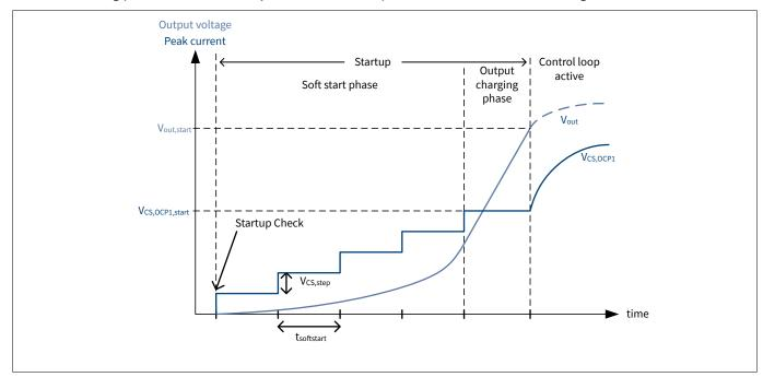
Figure 20 Flyback Startup Sequence
