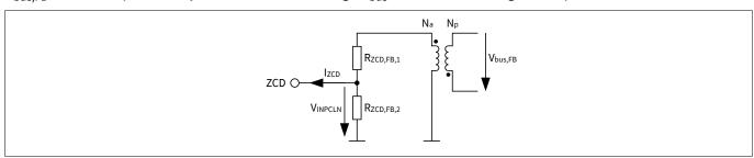
Figure 16 Voltage Sensing using ZCD Clamp Current
