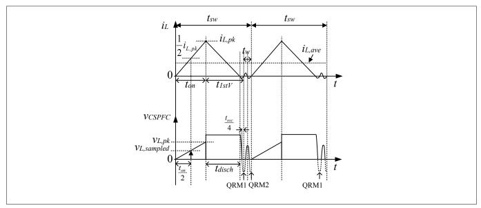
Figure 5 **PFC QRM2 Waveforms**
