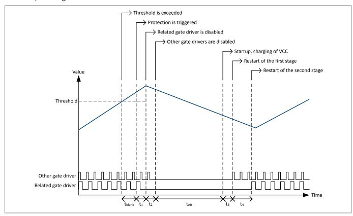
Figure 27 **Protection Reaction for auto-restart**
