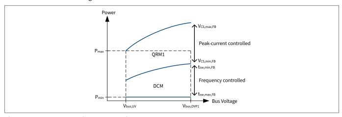
Figure 19 Flyback Multimode Operation Scheme
