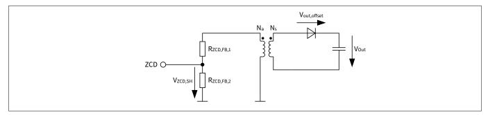
Figure 15 Primary Side Output Voltage Sensing using ZCD S&H
