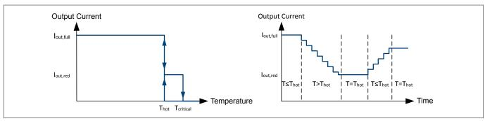
Figure 23 **Adaptive Temperature Protection**
