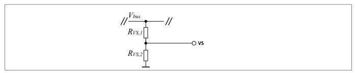
Figure 6 **Bus Voltage Sensing Schematic**
