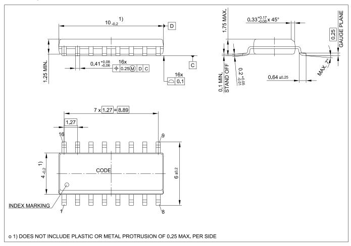
Figure 29 Package Dimensions for PG-DSO-16
