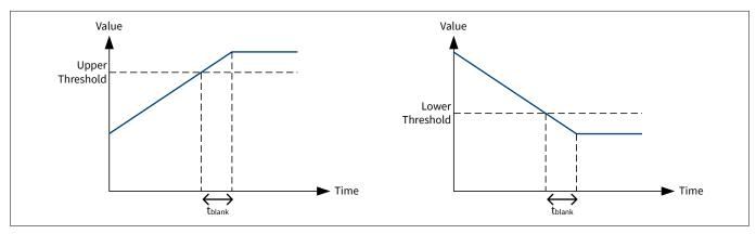
Figure 25 Blanking Times cause Excess of Threshold
