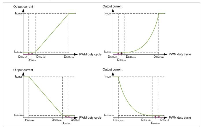
Figure 24 **Selectable Dimming Curves**
