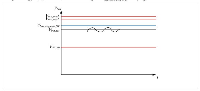
Figure 11 V<sub>bus</sub> protections
