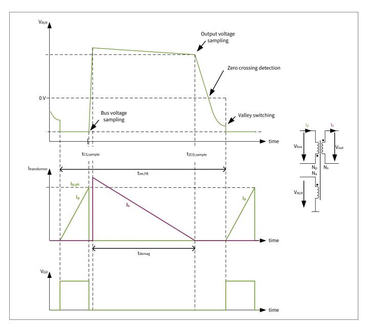
Figure 13 Typical Waveforms of a Flyback Converter
