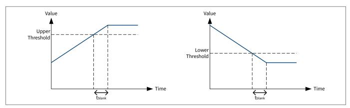
Figure 21 Blanking Times cause Excess of Threshold
