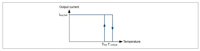
Figure 26 Temperature Protection
