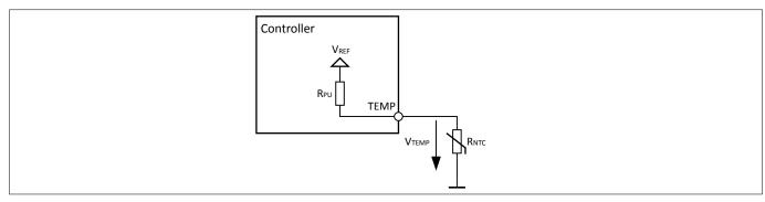
**External Temperature Sensing using NTC**
