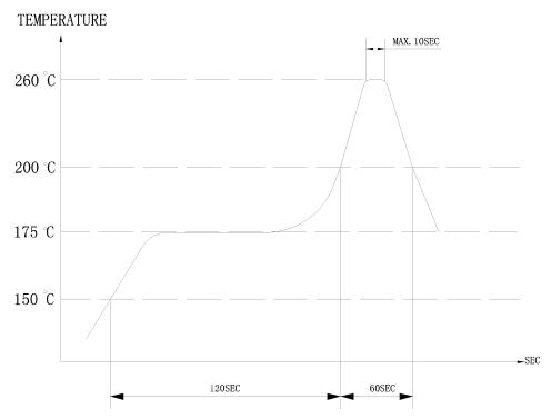
Heat resistant line (Used when heat resistant reliability test is performed) (2)Manual soldering Manual soldering temperature 350 °C within 5 sec.
