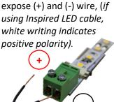
4 Taking note of (+) polarity of LEDs, insert flex strip into gap between black sliding latch and beige bridge piece.
