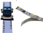
7 Strip cable back 14" to expose (+) and (-) wire, (if using Inspired LED cable, white writing indicates positive polarity)
