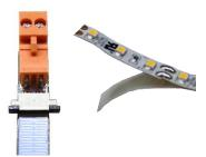
7 Strip cable back ¼" to expose (+) and (-) wire, (if using Inspired LED cable, white writing indicates positive polarity)
