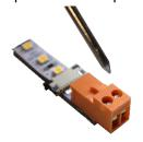
3 Peel back adhesive lining on LED strip
