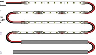
STEP 4: Close locking cap until the snap of the connector is heard. The snapping sound indicates the locking cap has been properly terminated.
