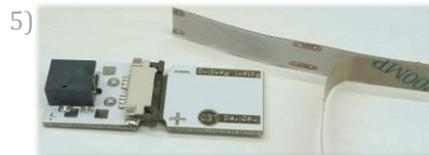
5) Now select the tiger paw that matches the polarity of the flexible LED strip end you would like to terminate. Peel back the adhesive liner on the LED strip about 1.5 inches. Please note that solder pads with a bump of solder on them cannot be terminated with this item.
