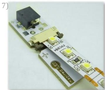
7) Make sure the LED strip is centered and fully inserted into the LED connector. You may need to hold the latch open with one hand so that the adhesive doesn't pull the latch closed prematurely.
