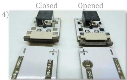
4) Also notice the LED connector - it opens for easy strip insertion and latches to secure the connection.
