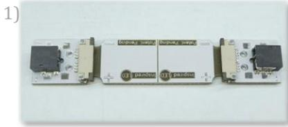
1) Tiger Paws come in pairs, to ensure that both ends of a flexible LED strip can be terminated.
