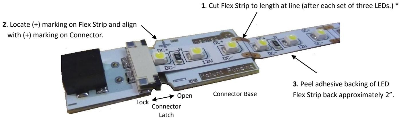
4. Holding latch open with thumb and forefinger slide Flex Strip fully into connector, slide latch to full lock position and press Flex Strip onto Connector Base.
