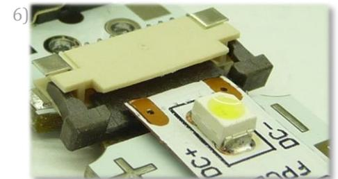
6) Insert the flexible LED strip into the **open** LED connector: *above* the sliding latch and *below* the beige top. Again, make sure that the positive side of the strip matches the positive side of the board.
