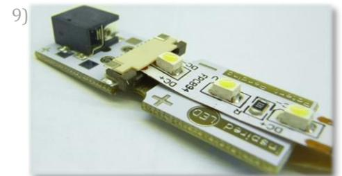
9) Reinforce the connection by pressing and sticking the flexible strip to the rest of the connector board.
