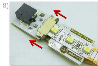
8) Secure the LED connector by closing the sliding latch. Again, the adhesive may want to resist. Your thumb nails are your friend here.
