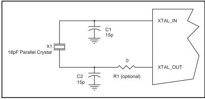
layouts. Slightly increasing the C1 and C2 values will slightly reduce the frequency. Slightly decreasing the C1 and C2 values will slightly increase the frequency. For the oscillator circuit below, R1 can be used, but is not required. For new designs, it is recommended that R1 not be used.
