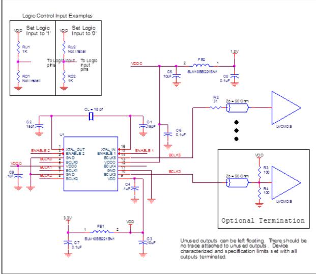
Figure 5. Schematic of Recommended Layout
