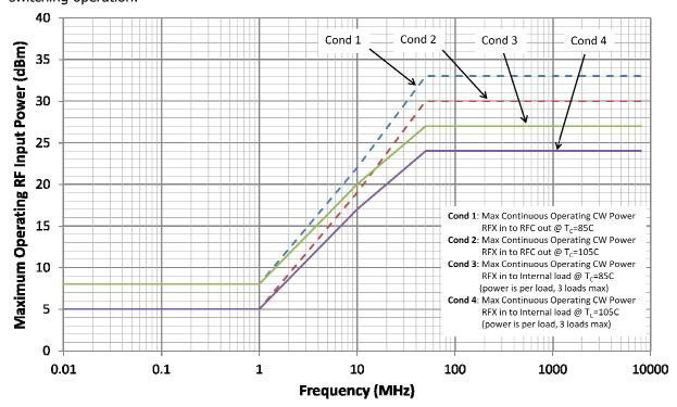
Figure 1 - MAXIMUM RF INPUT POWER VS. RF FREQUENCY
