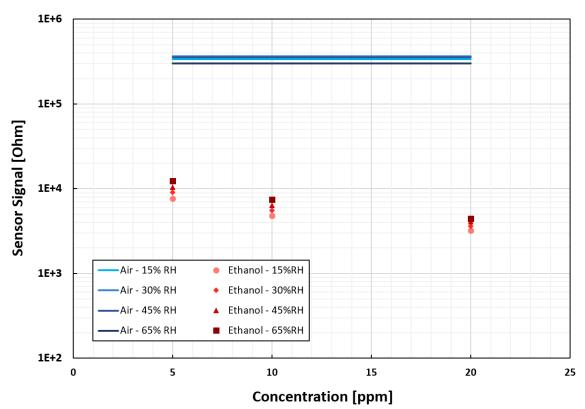
Figure 7. Humidity Influence at Three Different VOC Concentrations
