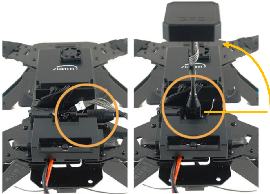
Figure 2. Raising the GPS Antenna Mast
