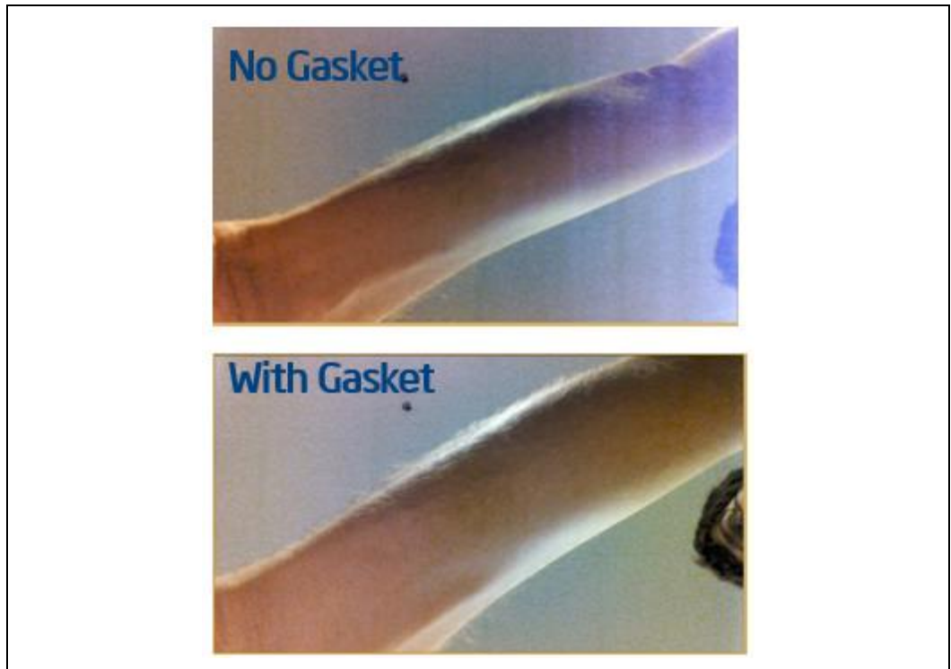
Figure 7-15. Example of Light Leakage Effects
