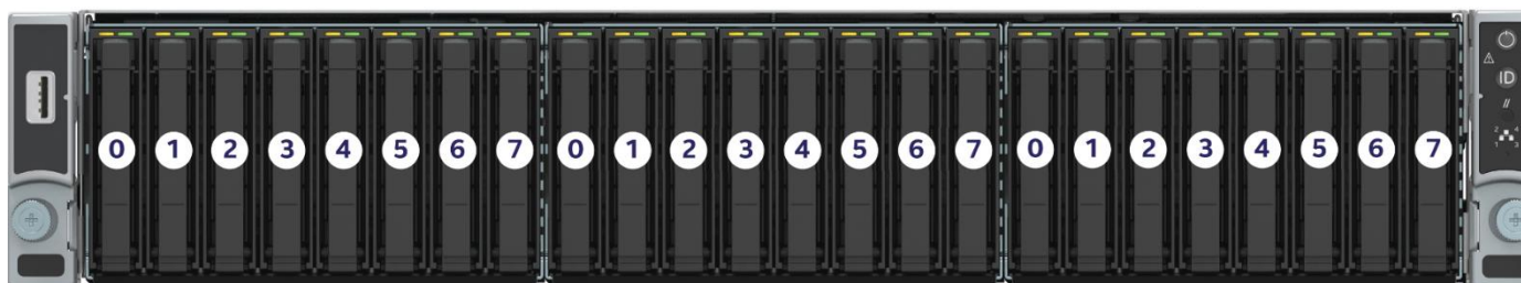
Figure 33. 2U 2.5" drive identification for each drive bay
