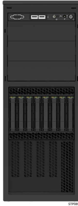
Figure 24. 8 x 2.5" hot-swap drive configuration (SATA/SAS 0-7)
