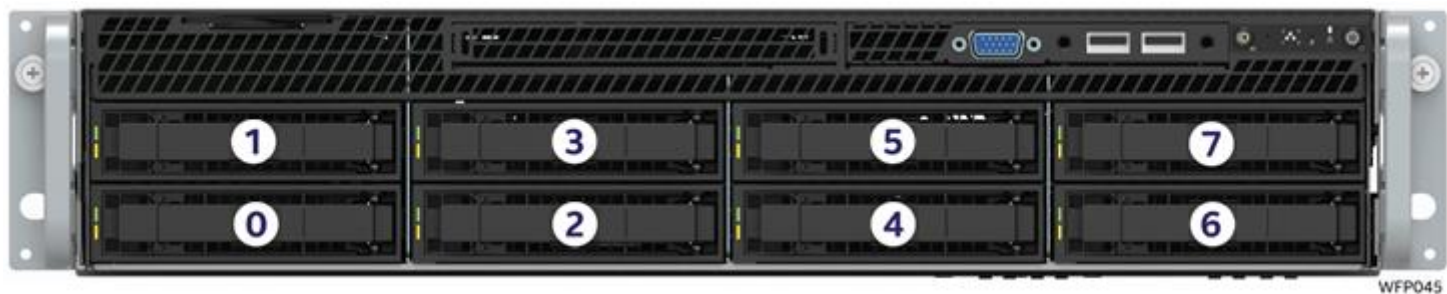
Figure 25. R2308WFxxx SAS/SATA backplane (no NVMe* support)
