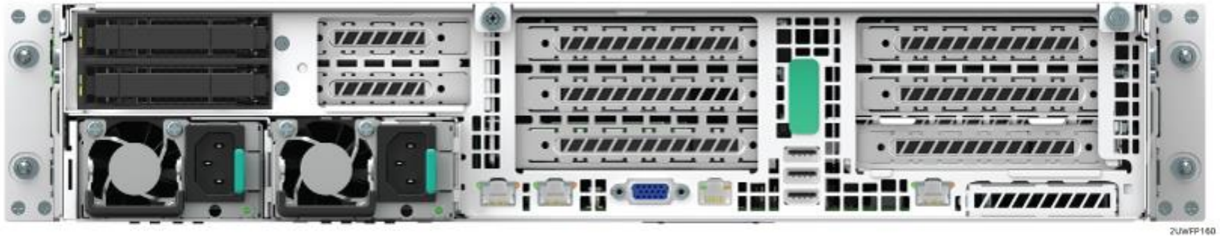
Figure 16. 2U System back panel with optional 2 x 2.5" hot swap drive bay
