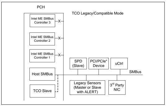
In TCO Legacy/Compatible mode the PCH can function directly with an external LAN controller or equivalent external LAN controller to report messages to a network management console without the aid of the system processor. This is crucial in cases where the processor is malfunctioning or cannot function due to being in a low-power state. Table 5-44 includes a list of events that will report messages to the network management console.
