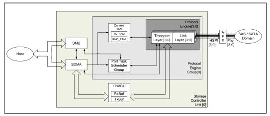
The single SCU-4 appears to the Driver as SCU[0]. There is a single Protocol Engine Group, PEG[0]. Within this Protocol Engine Group there are four Protocol Engines, PE[3:0], which connect to Phy[3:0]. There are four Port Task Schedulers (PTS), some of which are disabled depending on how the Driver configures it for Wide Port. Note that although the figure shows the SCU connecting to a SAS/SATA Domain, this could be direct-attached SAS or SATA disks.
