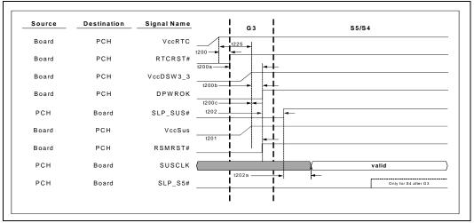
**Note:** VccSus rail ramps up later in comparison to VccDSW due to assumption that SLP\_SUS# is used to control power to VccSus.
