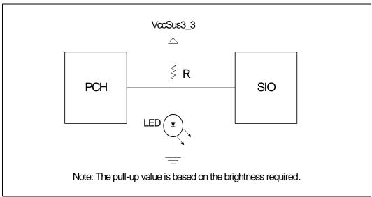
The anticipated usage model is that either the PCH or the SIO can drive a pin low to turn off an LED. In the case of the power LED, the SIO would normally leave its corresponding pin in a high-Z state to allow the LED to turn on. In this state, the PCH can blink the LED by driving its corresponding pin low and subsequently tri-stating the buffer. The I/O buffer should not drive a '1' when configured for this functionality and should be capable of sinking 24 mA of current.
