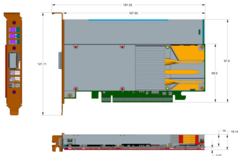
Figure 4. Acceleration Card - Standard Profile Bracket with Airduct
