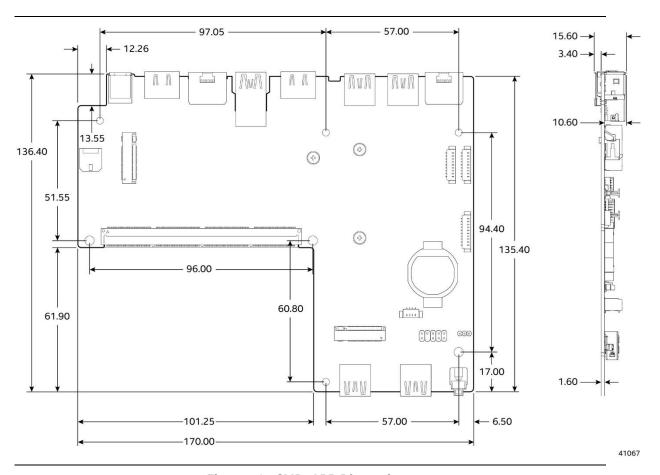
Figure 10. CMB1ABB Dimensions
