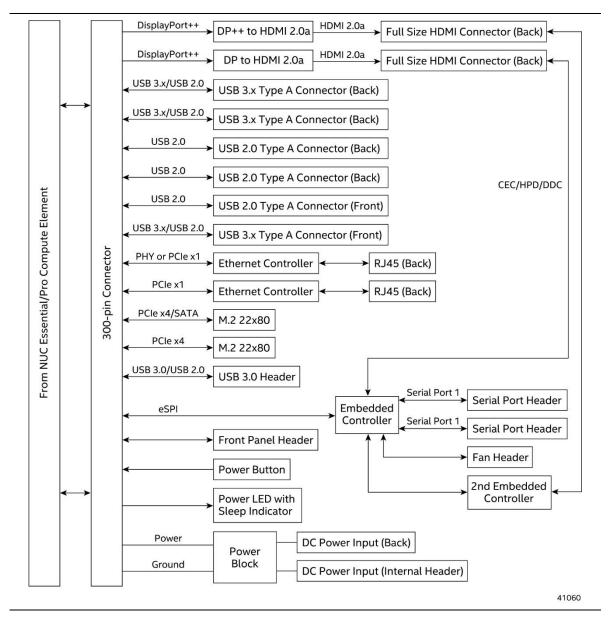
Figure 2. CMB1ABB Block Diagram
