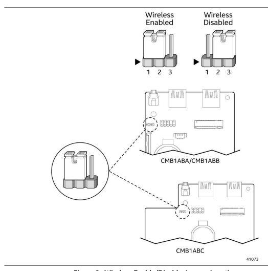
Figure 8. Wireless Enable/Disable Jumper Location
