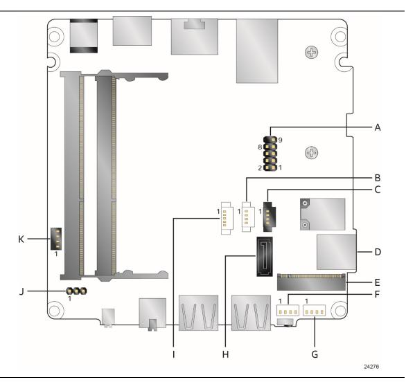
Figure 12. Connectors and Headers (Bottom)
