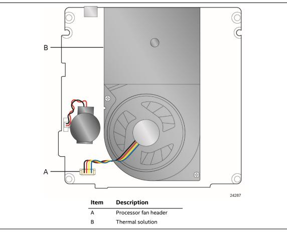
Figure 7. Thermal Solution and Fan Header
