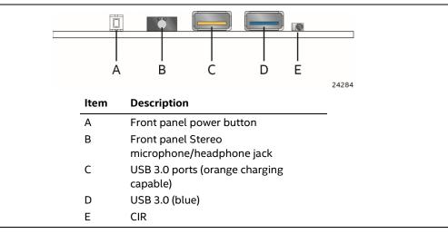
Figure 9. Front Panel Connectors
