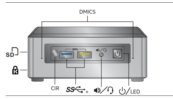
Figure 22. Intel NUC Kit NUC7i5BNH/NUC7i7BNH Features – Front
