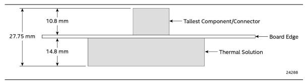
Figure 18. Board Height Dimensions
