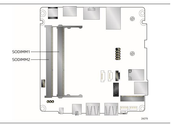
Figure 4. Memory Channel and SO-DIMM Configuration
