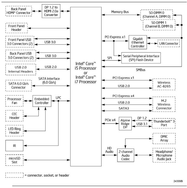
Figure 3. Block Diagram
