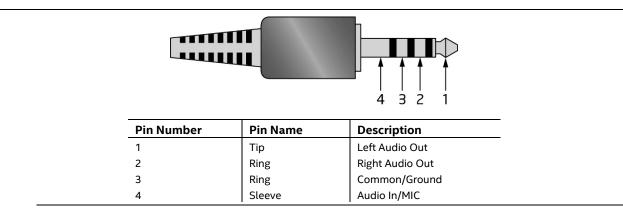
Figure 5. 4-Pin 3.5 mm (1/8 inch) Audio Jack Pin Out
