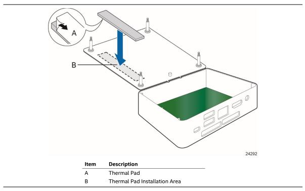
Figure 20. Installation Area of Thermal Pad for Intel NUC Kit NUC7i5BNK
