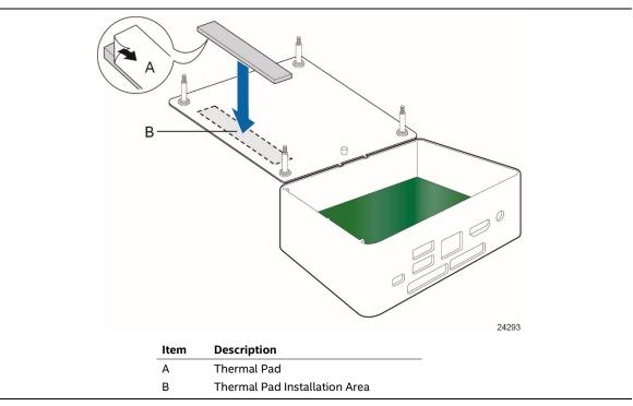
Figure 21. Installation area of Thermal Pad for Intel NUC Kit NUC7i5BNH/NUC7i7BNH
