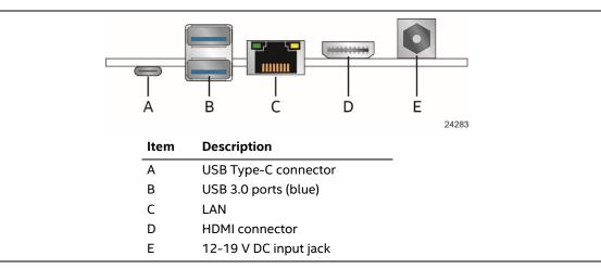
Figure 10. Back Panel Connectors
