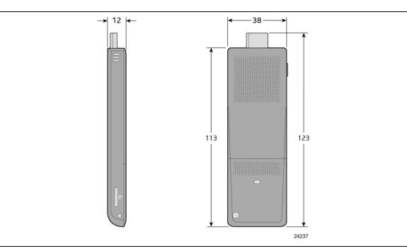
Figure 11. Intel Compute Stick Dimensions
