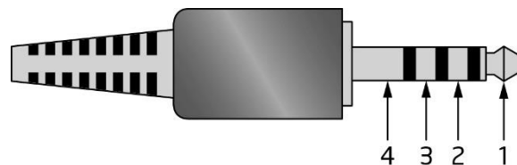
Figure 4. 4-Pin 3.5 mm (1/8 inch) Audio Jack Pin Out
