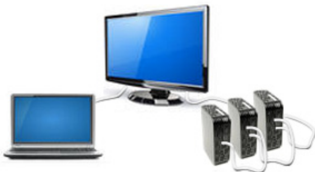
Figure 1. Thunderbolt™ cables expand a thin and light laptop to a high-resolution display and high-performance storage in a simple daisy chain.
