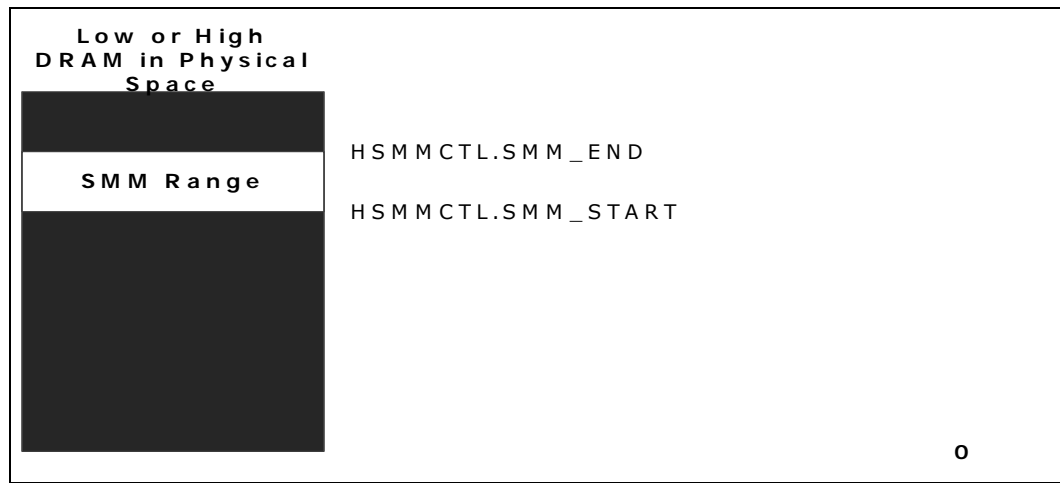
Figure 16. Physical Address Space - SMM Range
