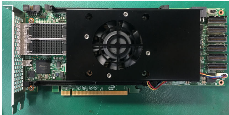
Figure 36. Air-cooled Heatsink Setup
