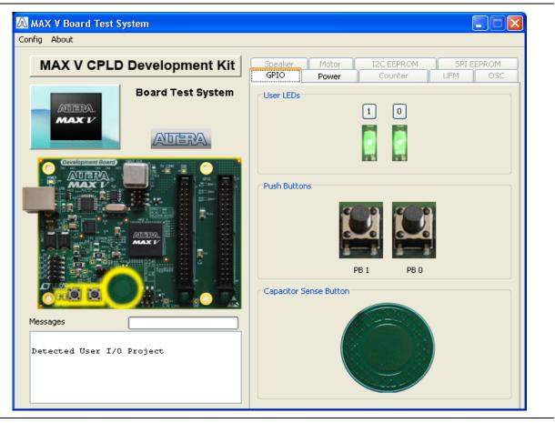
The following sections describe the controls on the GPIO tab.
