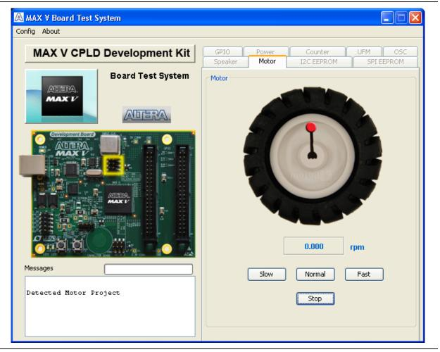
The following sections describe the controls on the Motor tab.
