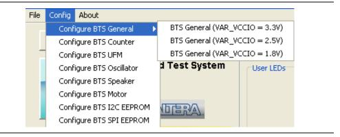
To configure the CPLD with a test system design, on the Config menu, click the configure command that corresponds to the functionality you wish to test.
