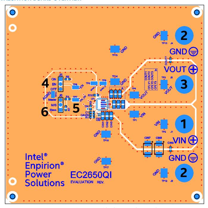
Figure 1: Evaluation Board (DIB) Features (Top View)
