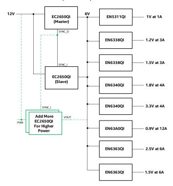
Figure 2: Parallel Operation with Master/Slave Mode
