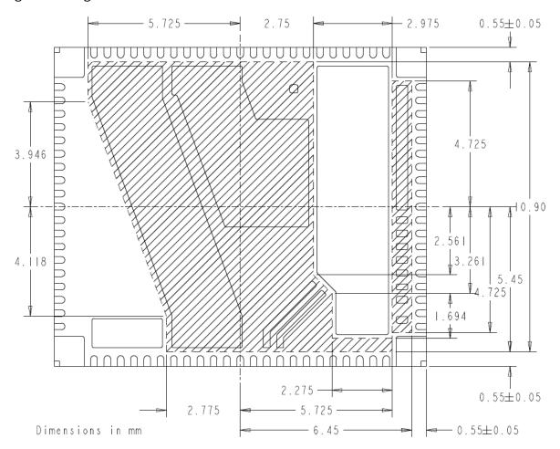
Figure 14: Lead-Frame exposed metal (Bottom View)
