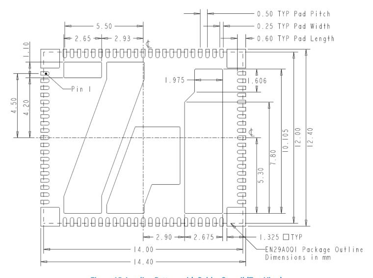
Figure 15: Landing Pattern with Solder Stencil (Top View)
