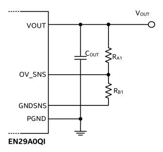
Figure 6: OVP trip-point external resistor divider
