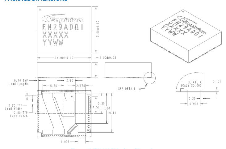
Figure 17: EN29A0QI Package Dimensions
