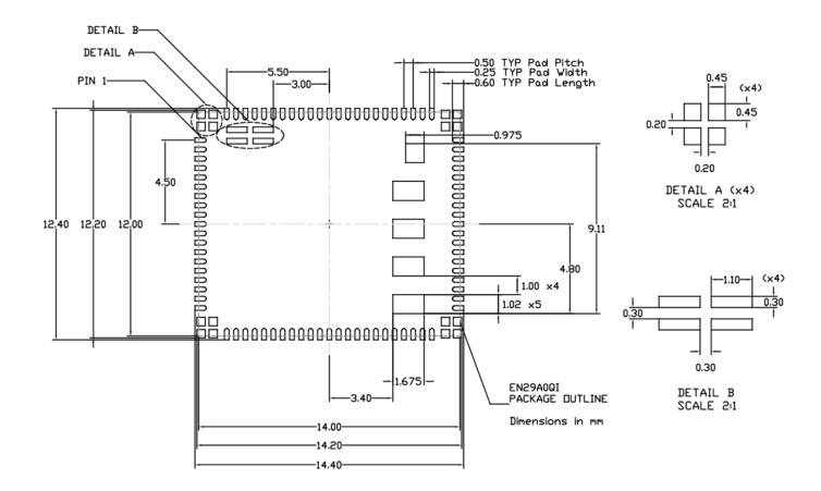
Figure 16: Solder Stencil Drawing
