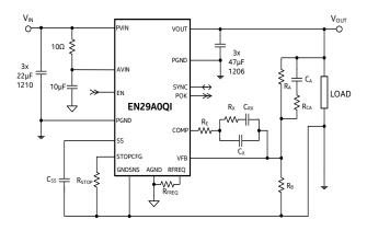
**Figure 1: Simplified Applications Circuit**
