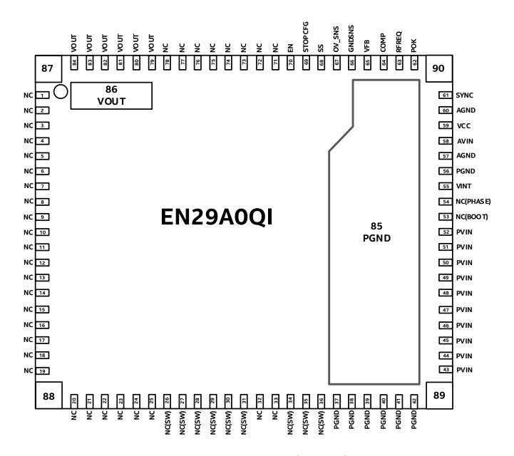
Figure 3: Pin Out Diagram (Top View)
