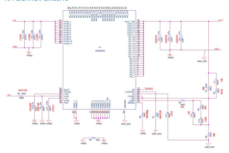
**Figure 9: Typical Application Circuit**
