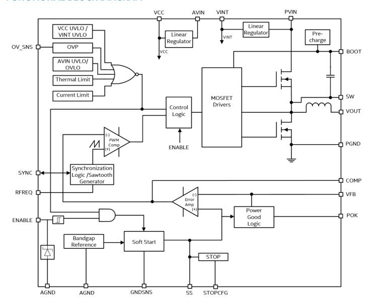
Figure 4: Functional Block Diagram
