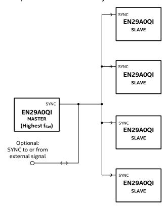
Figure 5: Frequency synchronization
