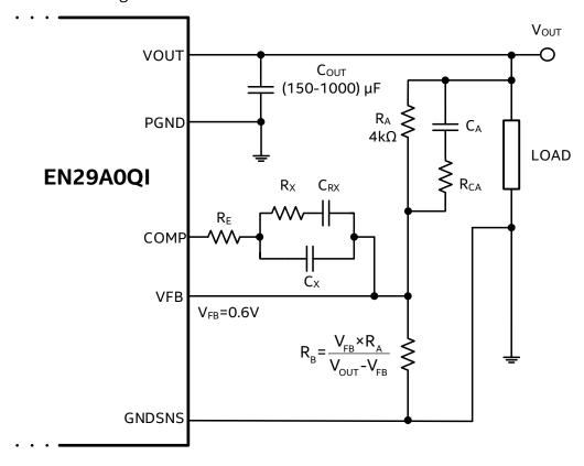
**Figure 7: VOUT Resistor Divider & Compensation Network**
