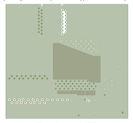
Figure 11: Inner Layer 2 – PGND
