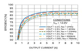
Figure 2: Efficiency at VIN = 12 V
