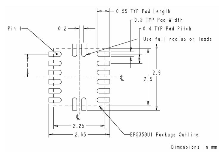
Figure 10: EP5358xUI Package PCB Footprint
