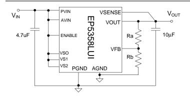
Figure 8: EP5358LUI using external divider
