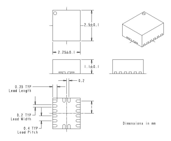
Figure 11: EN5358xUI Package Dimensions
