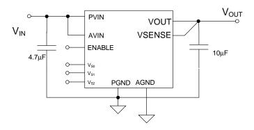
Figure 6: Application Circuit, EP5358HUI,.
