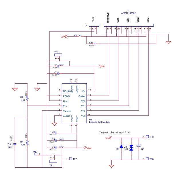
Figure 4: 3x3 Module Evaluation Board Schematic
