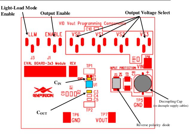
Figure 1. Evaluation Board Layout.
