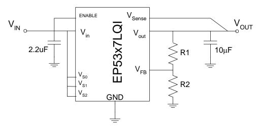
Figure 3. External divider schematic for the EP53x7LQL
