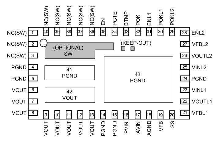
Figure 3: Pin Diagram (Top View)
