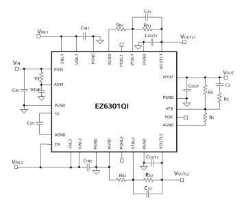
**Figure 1: Simplified Applications Circuit**
