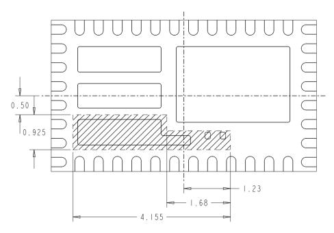
Figure 10: Lead-Frame exposed metal (Bottom View)
