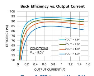
Figure 2: Efficiency at V<sub>IN</sub> = 5 V
