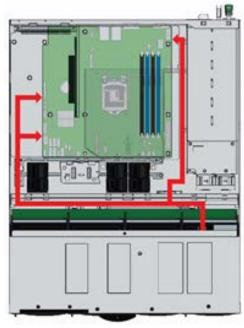
Figure 5. Intel® Server System R1000SPO Cable Routing
