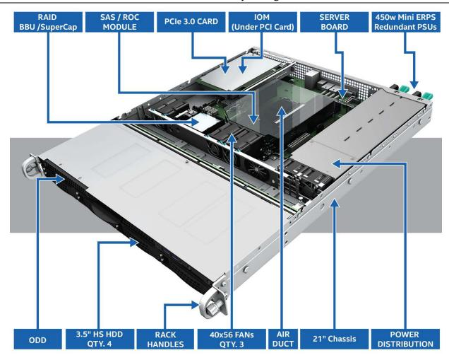
Figure 1. Intel® Server System R1000SPO Feature Set Identification
