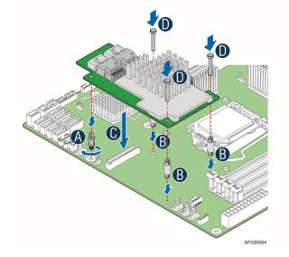
Figure 6. Installing Intel® Integrated SAS RAID Mudules
