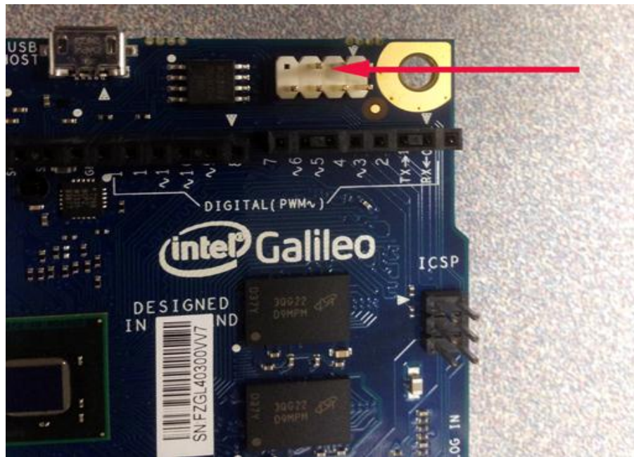
Figure 23. DediProg Header on the Target System
