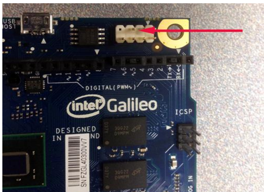
Figure 10. DediProg Header on the Target System
