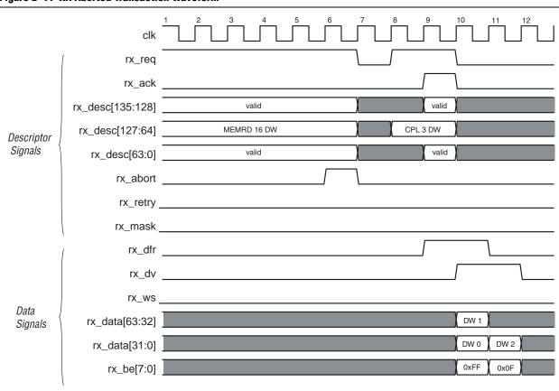
Figure B-7. RX Aborted Transaction Waveform
