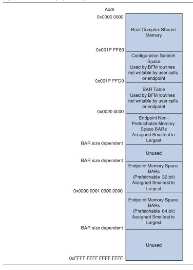
Figure 15–9 shows the I/O address space.
