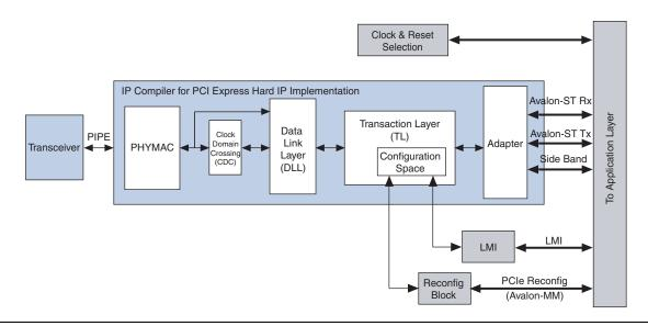
Figure 4-4. PCI Express Soft IP Implementation with Avalon-ST Interface to User Application
