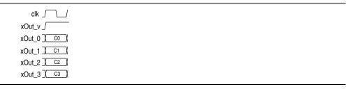
This result appears to be vertical, but that is because the number of cycles is 1, so on each wire there is only space for one piece of data.
