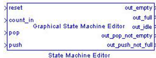
Figure 11-7. fifo_controller Block After Closing the State Machine Editor
