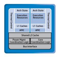
Intel® Core™2 Duo processor, based on Intel® Core™ microarchitecture, includes two complete execution cores, shared L2 cache, and intelligent power management features which deliver significantly greater performance-per-watt over previous-generation dual-core Intel® processors.
