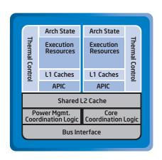
Intel® Core™2 Duo processors, based on Intel® Core™ microarchitecture, include two complete execution cores, shared L2 cache, and intelligent power management capabilities. These features deliver significantly greater performance-per-watt over previousgeneration dual-core Intel® processors.
