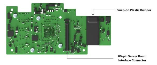
Figure 1. Intel® RMSP3AD160F RAID module layout
