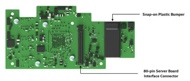
Figure 4. Intel® RMSP3CD160F RAID module layout
