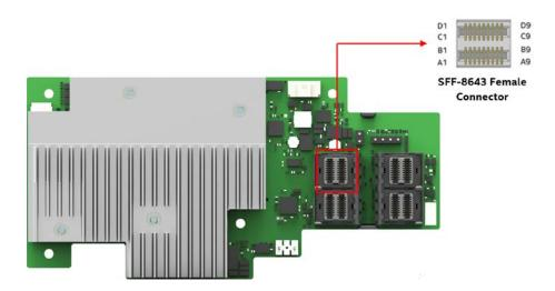
Figure 10. Intel® RMSP3AD160F RAID Module SFF-8643 connector
