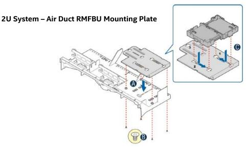
Figure 22. RMFBU assembly installation (example)
