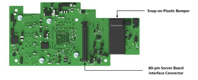
Figure 7. Intel® RMSP3HD080E RAID module layout
