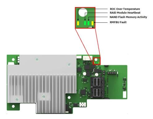
Figure 5. Intel® RMSP3CD160F RAID module LED description
