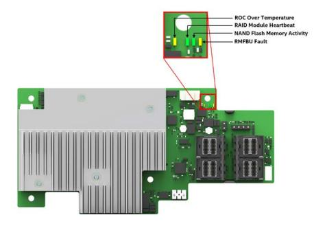
Figure 2. Intel® RMSP3AD160F RAID Module LED description
