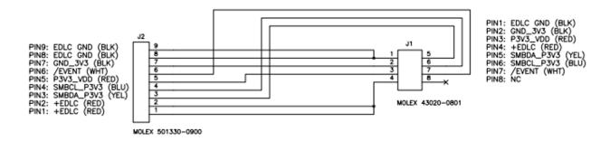
Figure 20. Extender cable pinout
