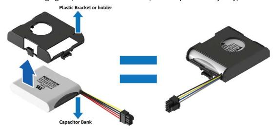
Figure 21. AXXRMFBU7 mounting assembly
