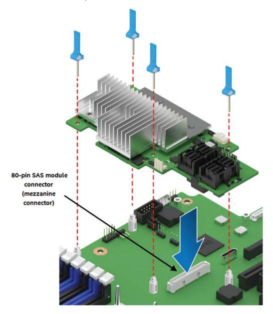
Figure 18. Intel® RAID module placement and installation
