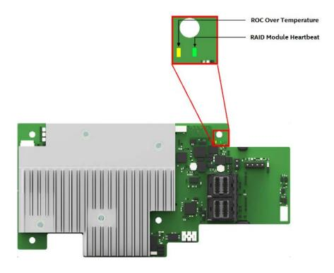
Figure 8. Intel® RMSP3HD080E RAID Module LED description
