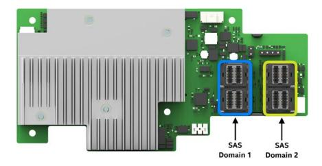
Figure 12. RAID module RMS3PAD160 SAS port domain identification
