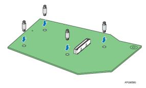
Figure 17. Barrel standoff placement and installation
