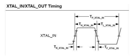
Figure 22. XTAL Timing Diagram
