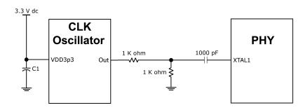
Figure 23. Clock Oscillator Schematic
