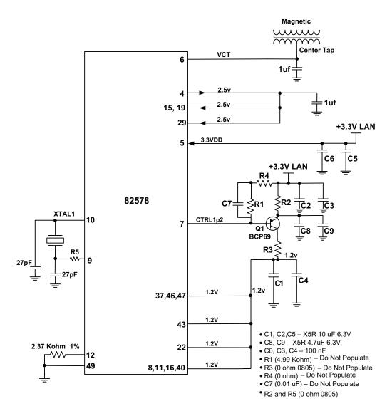
Figure 4. 82578 Power Delivery Diagram
