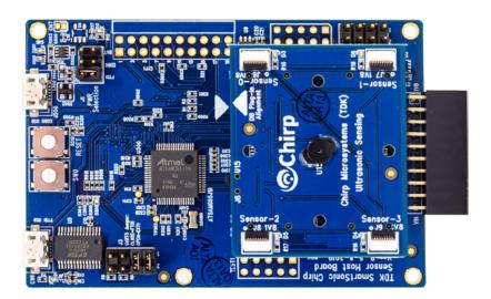
Part of the SmartSonic platform, the DK-CH101 is designed around Atmel's SAMG55 Cortex-M4 MCU, and can be used by developers for rapid evaluation and development of CH-101 based solutions. The DK-CH101 includes an on-board Embedded Debugger so external tools are not required to program or debug the SAMG55 MCU. The DK-CH101 includes an on-board Embedded Debugger so external tools are not required to program or debug the SAMG55 MCU.
