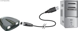
3. Connect the USB Type A connector of the USB cable from your USB device to the Type A port on the GUB231 or GUB431.
