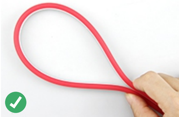
Face to the lighting surface and fold the strip. The minimum bending diameter is 80mm
