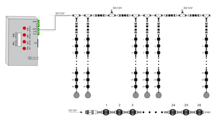
Attention: Input DC12V from start, Voltage drop to 0.5V on No.26 pcs ball on the end!
